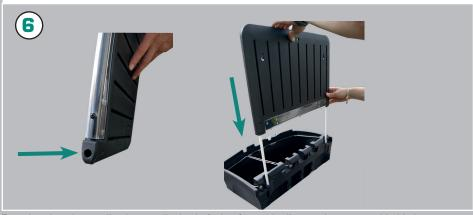
Ensuring that the acrylic signage display is facing forwards, line up the two moulded holes found on the underside edge of the sign with the 10mm support poles (as shown). Gently push downwards until located. **Please Note:** Do not force into place.
