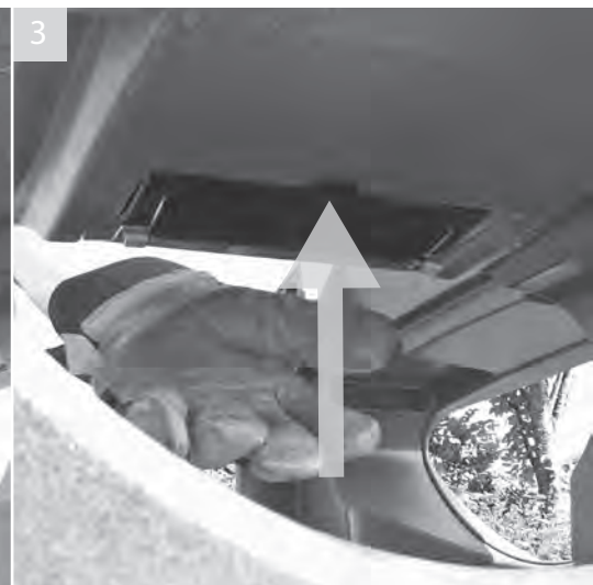
Once the contents of the ashtray has fallen into the liner release grip, the sprung hinge will return the flap to its closed position
