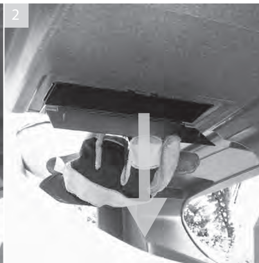
Pivot the ashtray flap downwards until it is vertical. Contents will fall into the liner below
