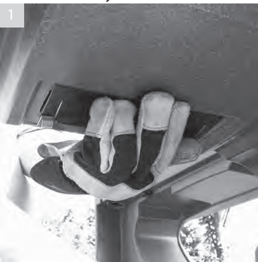
From door aperture reach inside the bin and grip the lip on the ashtray hinge flap
