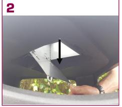
Pivot the ashtray flap downwards until it is vertical. Contents will fall into the liner below.
