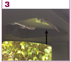
Once the contents of the ashtray has fallen into the liner release grip, the sprung hinge will return the flap to its closed position.
