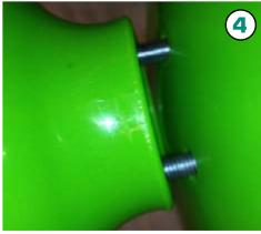
Align the eye moulding up then screw the first bolt and washer in a couple of turns. Then insert the second bolt and washer also tightening a couple of turns.
