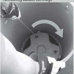
Using a stiff rod, depress locking pin on ballast cartridge, whilst pushing down twist bin body anti-clockwise, rotate until bin is free
