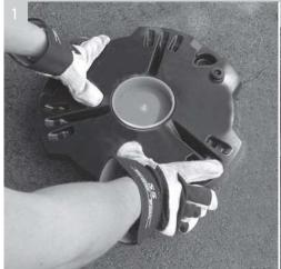
Position the ballast cartridge so that the locking Using chalk mark the position through the pin is at 45 in a clockwise direction from the direction that the lock on the bin will face
