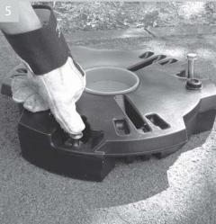
Drill 12mm holes in the three marked positions Re-position the cartridge over the drilled holes. Add washers to bolts and push through holes in cartridge locating into drilled ground holes
