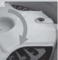
Twist bin body clockwise to lock. Locking pin will move beneath bin body until it reaches the locating hole where it will pop up and lock
