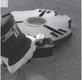
Use socket to tighten bolts, tighten to 22.0Nm torque for concrete. Tightening the bolts will
