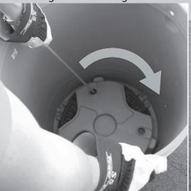
Using a stiff rod, depress locking pin on ballast Remove cap and Pour gravel into the cartridge cartridge, whilst pushing down twist bin body anti-clockwise, rotate until bin is free
