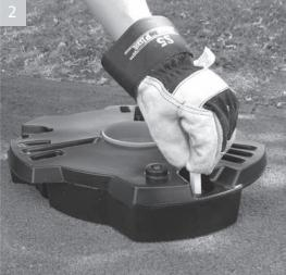
Using chalk mark the position through the three holes onto the ground bellow
