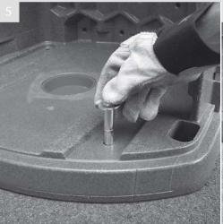
washers to bolts and push through moulded holes locating into drilled ground holes beneath
