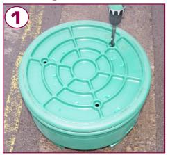
Using a hand drill, turn the bin base over and drill through the ground fixing locators as shown.
