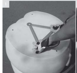
Remove hood and liner. Turn bin over and place the anchor plate in the centre of the bin through the three anchor plate holes and base. Orientate so a point faces the bin front
