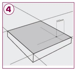
On the paving slab surface, make sure the marked positions are not within 100mm of the edge of the slab as cracking could occur.
