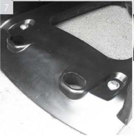
Drive the bolts in through the moulded holes unril the tops sit flat on the bin base with the washer between the bolt head and bin.
