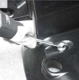
Use a spanner or socket to tighten the bolts.
