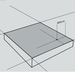
Check - if fixing to pavement check that the hole positions are not too close to the edge of the paving slab (min 100mm from edge if possible)
