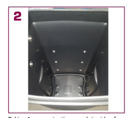
Taking 1 screw at a time reach in side of the 100L Envirobin. Tightening each screw by hand.
