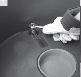
Use a spanner or socket to tighten the bolts
